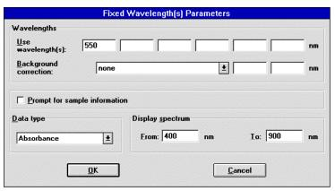
The diode array always collects the full spectrum since it contains a separate detector for every nanometer from 200 to 1100 nm. The upper left portion of the screen (shown above left) controls the display of the data. Selecting fixed wavelengths gives the dialog shown at right. As well as displaying the spectrum for the selected range, absorbance values will be tabulated for the selected wavelengths. Click on the setup button to return to the dialog box.
